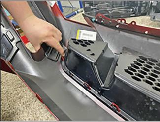
Once the clips are released, pull to remove the original grille from the front bumper cover panel.
