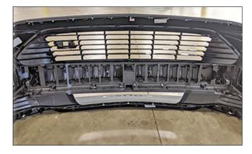
3. Position the front bumper cover to the vehicle. Reinstall the two (2) front bumper cover bolts using a 5.5 mm socket. Reinstall the six (6) front bumper cover bolts using a 8 mm socket.
