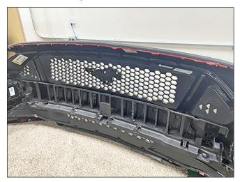
2. Using a trim tool, remove the three (3) top clips and the three (3) bottom clips from the front bumper cover support panel.
