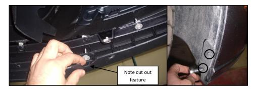
4. Install the closeout panel. The lower closeout panel must be positioned between the factory splitter and the new chin splitter.
