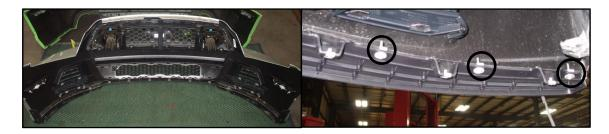
2. Install the remaining six (6) J-Clips (W704823-S439) found in the hardware kit onto the new splitter in the areas shown below.
