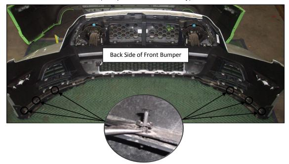
5. Depress the six (6) tabs protruding through the slots in the lower area to remove the factory splitter.
