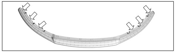
12. With a suitable drill and a 1/8 IN drill bit, drill the six (6) marked holes. With a 1/4 IN drill bit, drill the six (6) pilot holes open to 1/4 IN. Install six (6) J-Clips (W704823-S439) from the hardware kit onto the six (6) newly drilled holes (right side shown below, left side similar).
