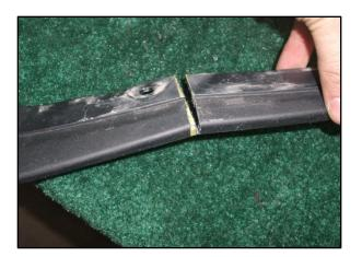
5. Using a pneumatic saw, cut along the lower body line as illustrated. Stop at the edge to retain the turned up mounting feature.
