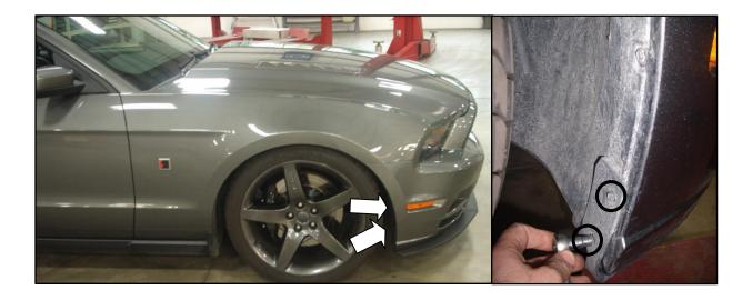
3. With the vehicle properly supported, access the underside of the engine bay. With an 8mm socket and ratchet, remove the front six (6) closeout panel fasteners and discard. Remove the remaining eleven (11) 7mm closeout panel fasteners and save for reinstallation. Remove the closeout panel.
