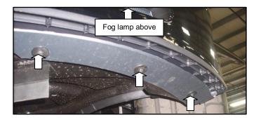
6. Install the remaining six (6) (W715060-S439) screws found in the hardware kit into the front portion of the closeout panel as illustrated below. Torque to 5 Nm (44 lb-in).
