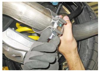
5. Place the band clamp (10-0338) over the exhaust tip and slide the tip over the muffler. Torque the band clamp to 30 Nm once the tip is in position.
