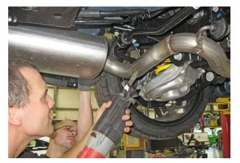
3. With the exhaust pipe cut, slide the hanger out of the rubber mount and remove the muffler/tip assembly from the vehicle.
