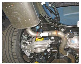
2. Cut the LH and RH exhaust pipes at the locations marked in step 1 using a reciprocating saw with a metal blade.
