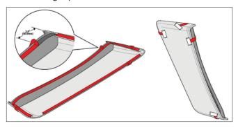
6. Install the side scoop onto the body side using the directions on the template. Do not allow the exposed double-sided tape to adhere to the sheet metal until the side scoop is properly aligned, then press down.
