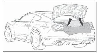
Carefully cut out the LH and RH inner drill templates from the larger template sheet (1315-SPLRTMPL). 6. Align the LH and RH inner template and secure to the inner sheet metal with masking tape, as indicated.
