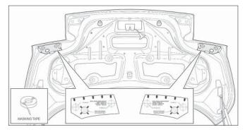
Create four (4) access holes in the trunk's inner sheet metal by center punching four (4) hole locations, two (2) per side. Drill each center punched location with a 1/8" drill bit. Enlarge each 1/8" hole with a 1.0" hole saw.
