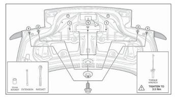
Re-install the two (2) OE rubber hole plugs removed in step 3. Install four (4) new 1.0" rubber holes plugs into the access holes drilled in Step 7.
