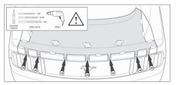
12. Test fit the rear spoiler. Align the five (5) studs on the rear spoiler through the holes drilled into the trunk lid. Secure the rear spoiler to the trunk lid with masking tape.
