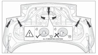
14. If the fasteners and holes are not aligned, remove the rear spoiler and use a round file to adjust the holes in the trunk lid outer sheet metal accordingly.
