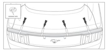
Open the trunk lid and inspect each of the seven (7) mounting holes. Confirm that the rear spoiler fasteners are properly aligned with the holes drilled in the trunk lid outer sheet metal.
