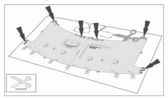
Install the trunk lid outer sheet metal drill template. With the trunk lid closed, align the large outer drill template onto the outer sheet metal of the trunk lid as shown. Secure template to trunk lid with masking tape.
