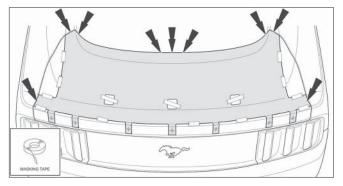
Drill seven (7) rear spoiler mounting holes. Center punch the seven (7) hole locations indicated on the template. Drill each center punch location with a 1/8" drill bit. Enlarge each 1/8" hole to the size indicated on the template. Note that the center hole should be enlarged to 5/16" while the other six (6) holes should be enlarged to 3/8".
