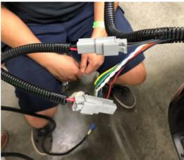
14. Zip tie and tape the harness together. Re-attach the electrical connector to the taillight and re-install the taillight using the two (2) screws previously removed. Torque to 5 Nm.
