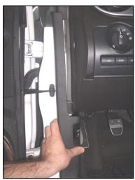
9. Un-clip the plastic carpet retainers from the driver side rocker panel to expose the vehicle wiring.
