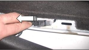
7. Unfasten, but do not remove, the driver side rear quarter trim panel. Locate and remove the trim pin fastening the panel. Grasp and pull the quarter trim panel outward to unfasten it from the driver door opening.
