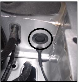
10.b. Pass the intermediate harness through the firewall and into the engine bay. Seat the grommet into the open port on the fire-wall.
