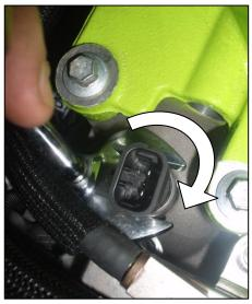
12.b. Following factory wiring, route the harness along the back of the engine to the passenger rear side of the intake manifold. Plug the connector into the switch installed in the previous step.
