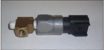
12.a. Install the switch and fitting into the port where the boost gauge fitting was removed in step 10.a. Torque the fitting to 12 Nm. Orientate the fitting so the open port is pointing toward the left-rear of the vehicle.
