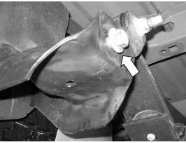
2. 2018-2020MY:Position the new catalyst pipe adapter flange into place against the catalyst pipe and loosely install the two (2) take-out fasteners to hold it in place.
