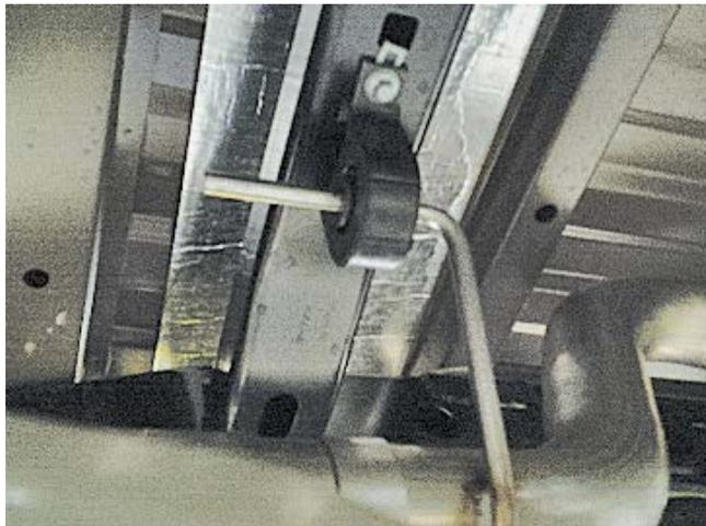
4. Remove the intermediate pipe and resonator from the vehicle.
