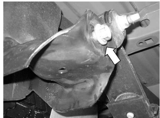
2. 2018-2020MY: Position the new catalyst pipe adapter flange into place against the catalyst pipe and loosely install the two (2) take-out fasteners to hold it in place.
