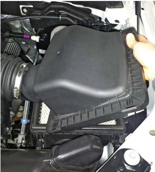
8. Remove the clean air tube from the vehicle.
