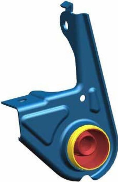
8. Locate (2) washers – 3/8" X .406" ID X 0.812" OD (11101304). Place them in between the modified bracket and the frame of the vehicle. Reinstall the modified exhaust hangers with the takeoff flange bolts. Torque to 25 Nm. (18lb.ft).
