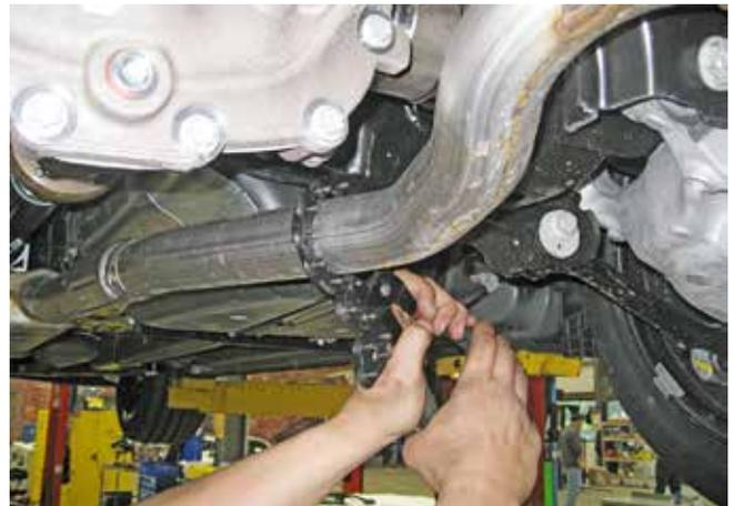
3. Remove the two (2) 13 mm bolts that retain the exhaust hangers on the IRS sub frame. Push up on heat shields.
