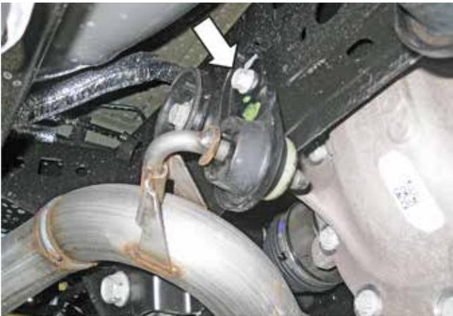
4. Remove electronic actuator, flange nuts, spring, and backing plate from mufflers to be removed. Set aside to be used later for install on Roush active valve assemblies.
