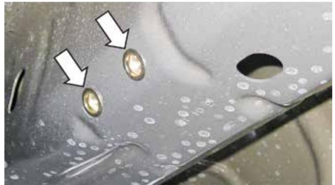
5. Install the two (2) supplied exhaust hangers (P/N: 1315-5A261 and 1315-5G298) and four (4) bolts (P/N: W500224) as shown below. Torque to 18 lb-ft (25 Nm).
