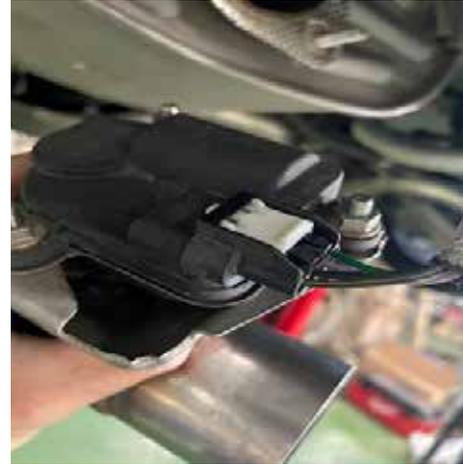
2. Disconnect wire harness from electronic actuators, Using a suitable exhaust pipe cutting tool, cut completely through the stock exhaust in the two (2) locations shown below. Unhook each exhaust hanger from the sub frame and remove each muffler assembly by sliding the inlets down and forward to extract the rear exhaust hangers from their mounts.
