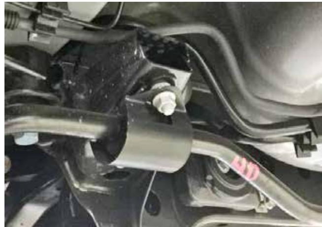
2. Locate the template onto the rear chassis sub frame as shown in the pictures below and mark the drill holes with a center punch. Use the same template to mark the holes on both the RH and LH sides of the vehicle.
