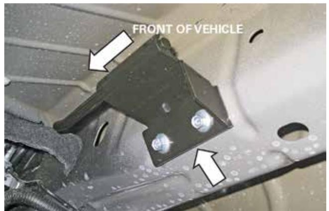
4. Deburr the drilled holes and apply automotive clear coat. Install four (4) rivet nuts (P/N: 95105A191) using the supplied bolt and nut from the rivet nut installation kit (P/N: R1315-5231HWK). Insert the nut onto the bolt and thread the bolt into the rivet nut. Hold the nut with a 17 mm wrench and tighten the bolt nut with a 10 mm socket until the rivet nut is fully seated.
