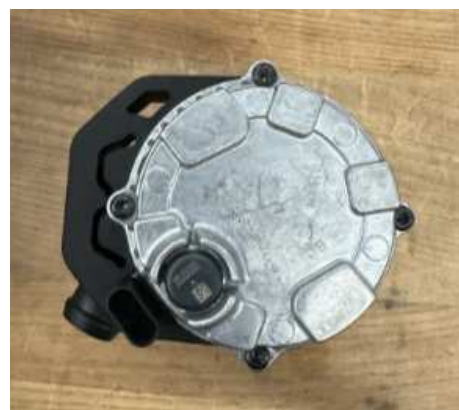
Intercooler pump sub-assembly_Bottom View
