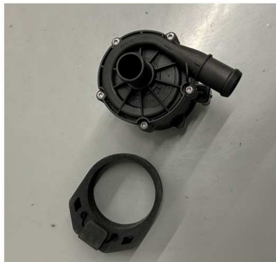
Intercooler pump and grommet facing up orientation
