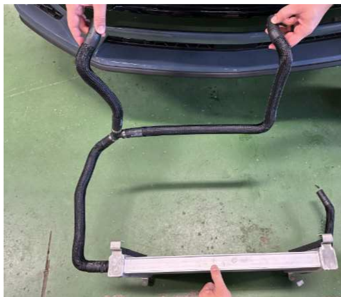
Top View Orientation - LTR Sub-Assembly
