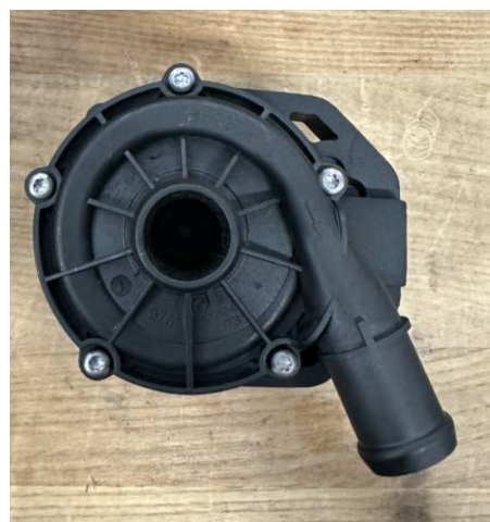
Intercooler pump sub-assembly_Top View
