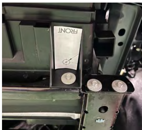
Driver Side template location
