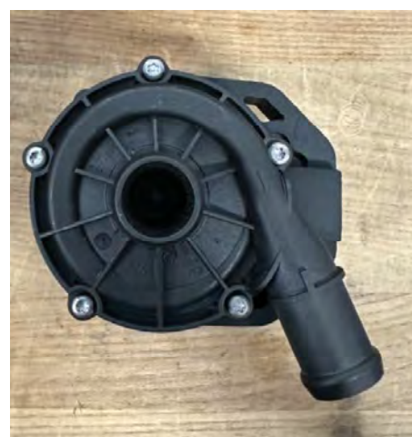
Intercooler pump sub-assembly_Top View
