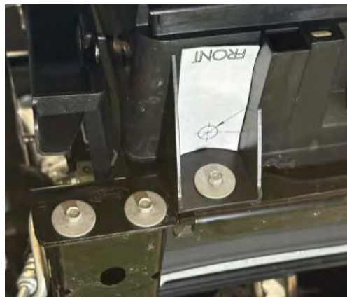
Passenger Side template location
