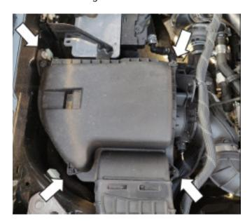
Remove the factory lid by using a small screwdriver or non-marring tool by inserting it here and twisting to release tension clips.
