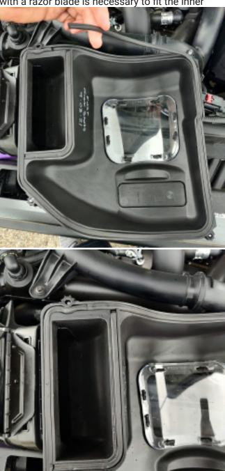
3. Wipe the lid with alcohol and install the ROUSH Badge (PT00041667) onto the air box lid by removing the backing tape and applying as shown.
