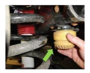
12. Use 10mm socket to remove factory mount from the frame. NOTE: Set aside Jounce Cup for Re-work.
