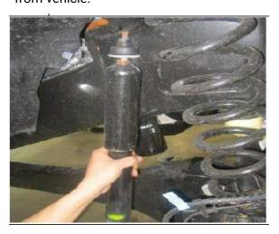
7. Transfer over upper rubber isolator and install new springs (9285). Be sure to align the spring locators on upper and lower mounts.
