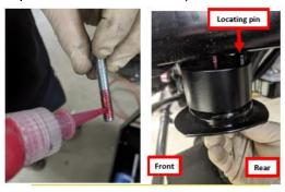
16. Tighten fastener to secure Front Jounce bumper assembly with Roush-modified cup. Torque fastener to 37 Nm and apply UV Mark. Reinstall rubber jounce bumper by pushing onto cup. Assembly will look as shown below.
