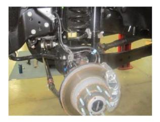
4. Remove upper shock nut, washer, and bushing on both sides of vehicle with 21 mm socket wrench. Discard hardware.
