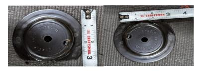
14. Assemble jounce bumper with modified jounce cup and spacer. (NOTE: 1818 will be etched into the part to identify it as the one to use)
