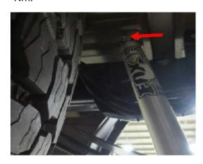
26. Fasten shocks at lower location with nut and bolt and 18mm and 21mm socket wrenches. Torque to 150 Nm.
