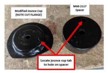
15. Apply Loctite 271 to M8 bolt before install. Install assembly on frame so cut flange faces outside of vehicle (pin on spacer will locate to rear).
