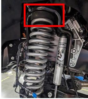
Install new shocks (986-24-098) and fasten lower bolts and flange nuts with 18mm socket wrench. Torque to 150 Nm.
