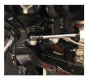
20. Torque bolts to 90 Nm for 19mm bolt and 80 Nm for 15mm bolt.
