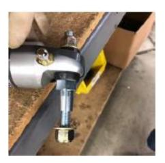
19. Apply Loctite 262 on both the bolts and loosely install the steering stabilizer on linkage on the driver side. Adjust the axle and install on the passenger side.
