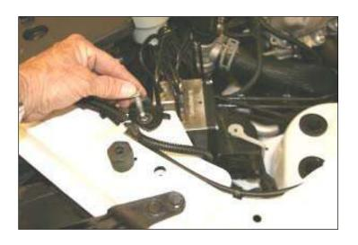
6. With a 10mm socket, remove and save the bolt that holds the factory anti lock brake bracket as shown.
