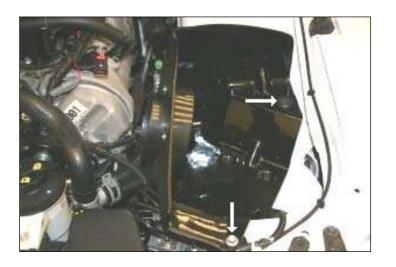
9. Install the <u>Cool Air Dam Assembly</u> pins (on bottom) into the factory grommets from Step #4. Reinstall the bolt from Step #3 using new <u>Fender Washer</u> into the inner fender. Reinstall the bolt from Step #6 into the anti lock brake bracket.
