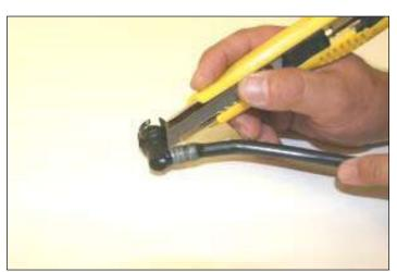
17. **VERY CAREFULLY!!!** With a razor knife, cut the plastic tube away from the factory ends of the breather tube assembly as shown.
