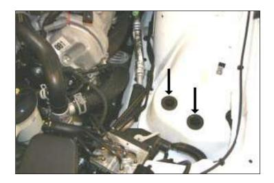
4. Remove the complete factory air inlet assembly. (Note: Make sure the two factory grommets remain in the lower air box support.)
