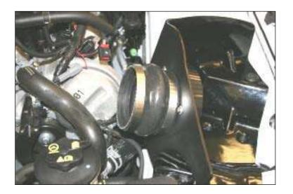
10. Install the <u>Hump Hose</u> onto the <u>Filter Adapter</u> with one <u>#64 Hose</u> <u>Clamp</u> and tighten. Place one <u>#64 Hose Clamp</u> loosely onto the <u>Hump Hose</u> as shown.
