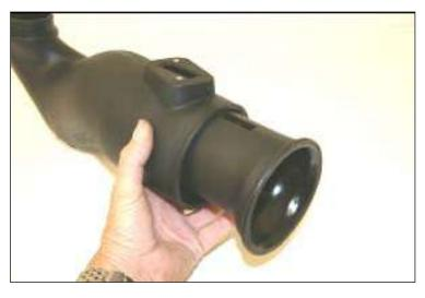
12. Insert the <u>Tube Insert</u> into the <u>ROUSH Intake Tube</u>, aligning the slots as shown.
