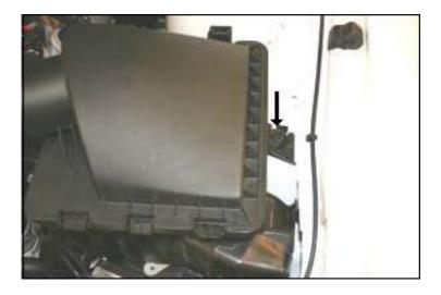
3. With a 10mm socket, remove and save the bolt that holds the factory air box to the fender.
