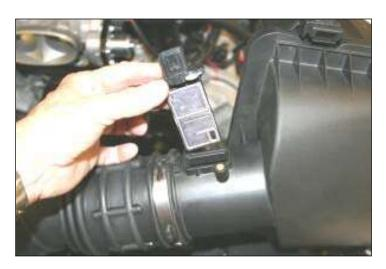
5. Using the provided #20 Torx Bit, remove the mass air flow sensor from the factory inlet air tube. (Save the mass air flow sensor for later use.)
