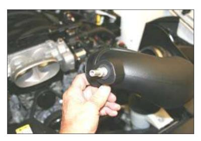
11. Install the <u>Grommet</u> into the <u>ROUSH Intake Tube</u> and then install the <u>Aluminum Fitting</u> into the <u>Grommet</u>, as shown, tapered end first.
