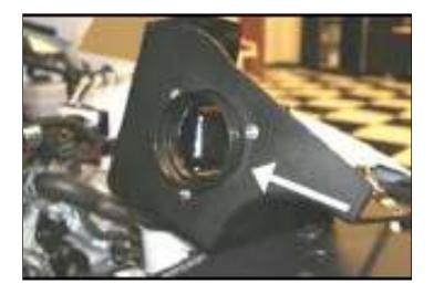
7. Install the <u>Filter Adapter</u> into the <u>Cool Air Dam</u> as shown, using three <u>1/4"-20 x 1/2" Button Head Bolts</u> and three <u>1/4" Flat Washers</u>.
