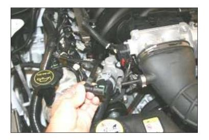
1. Disconnect battery negative cable. Remove the breather hose assembly from the vehicle by pushing in on the green plastic tabs to release each fitting. (Save breather hose for later use.)
