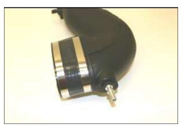
14. Install the <u>Oval Coupler</u> with one #72 Hose Clamp and tighten. Place the second #72 Hose Clamp loosely onto the <u>Oval Coupler</u> as shown.
