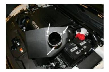
7. Install the Filter Adapter to the inside of the Cool Air Dam, using the three ¼"-20 Hex Bolts and ¼" Flat Washers as shown
