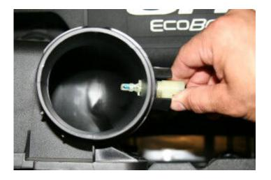
9. Remove the air temperature sensor from the factory air box by rotating the sensor ¼ turn counter clockwise and pulling outward.
