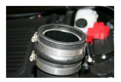
8. A) Install the Hump Hose, large side first onto the Cool Air Dam tube. Loosely install the #56 Hose Clamp on the small side of the Hump Hose, and the #60 Hose Clamp on the large side.
