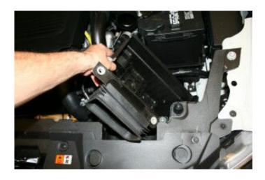
5. Remove the factory air box assembly from the vehicle.
