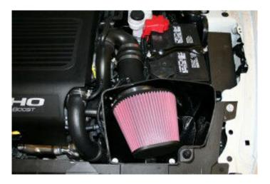
12. Install the ROUSH Premium Filter onto the adapter and tighten the clamp.
