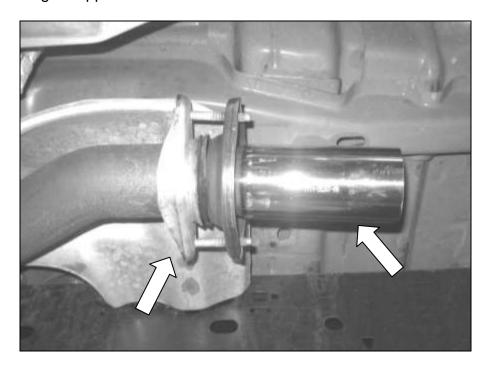
3. Position the new muffler outlet axle pipe (1111-5C262 if Rear Exit, 1113SE-5C262 if Side Exit) into position and install the steel hanger brackets into the factory rubber hangers. Orient the pipe such that the flared end faces forward in vehicle.
