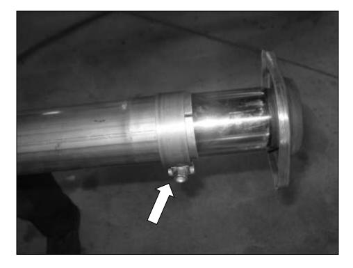
9. Insert one (1) 3" clamp (R12060012) over the end of the intermediate pipe and insert the intermediate pipe into the muffler. Position the clamp on the pipe joint and loosely secure.
