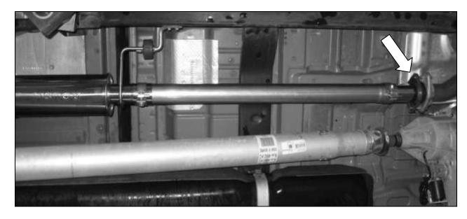
11. Install one (1) 2.5" clamp (R12060014) onto each of the exhaust tips and slide the tips (1111-5230TIP if Rear Exit, 1113SE-5230TIP if Rear Exit) onto the ends of the Y-pipe (1111-5255 if Rear Exit, 1113SE-5255 if Side Exit). Position the clamps on the pipe joints and loosely secure the clamps.
