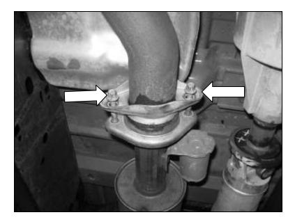
2. Loosen the clamps, which secure the intermediate pipe and resonator to the muffler and tail pipes.
