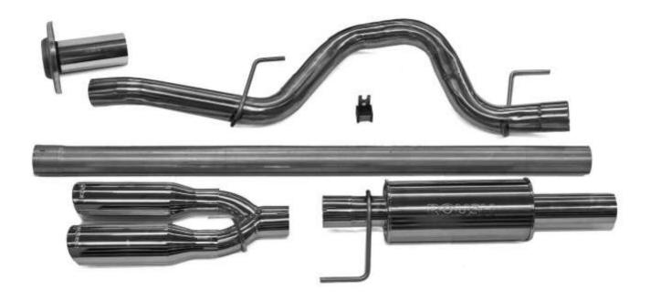
Note: Rear exit exhaust system displayed; side exit exhaust content similar.
