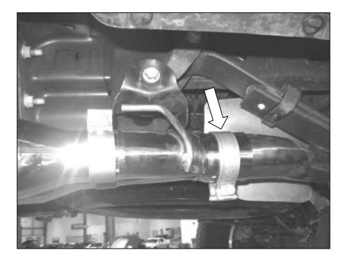
13. Insert the Y-pipe hanger into the hanger bracket (1111-5A204). It is important to note the orientation of the bracket as it will hang underneath the suspension bracket.
