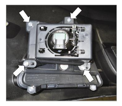
11. Remove the four (4) screws and the fog lamp mounting bracket.
