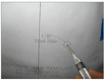
4. Remove the template and drill the marked locations to a 1/8" pilot hole, working your way up to a 3/8" pilot hole.
