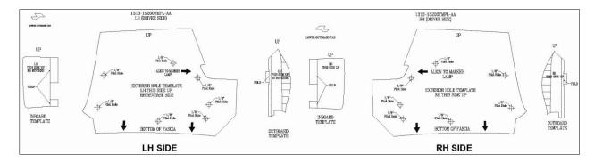
2. Position the exterior hole template on the bumper cover, align the marker lamp provision, align the bottom of the template to the bottom of the bumper cover edge and tape in position.
