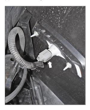
7. Pull outward to unsnap the LH and RH sides of the bumper cover.
