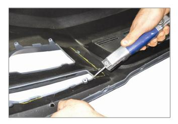
8. Deburr the cut edges on the bumper cover and repeat steps 2 through 8 for the opposite side. Once both sides of the bumper cover have been cut, test fit the fog lamp bezels for proper installation.
