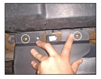
**NOTE:** After drilling the holes, apply commercially available clear coat such as Motorcraft<sup>®</sup> (P/N: PM-19500-600) to the bare metal surfaces.
