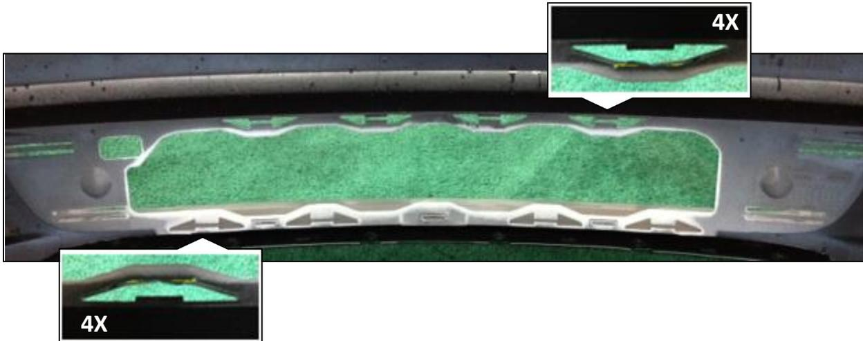
7. Apply adhesion-promoter to the surface where tape is to be applied. Apply on the lip of the part, at the parting line. Allow to set for 60 seconds.
