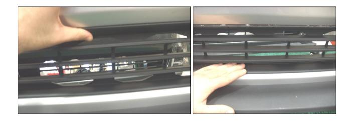
• To install the lower valance panel, reverse the removal procedure.
