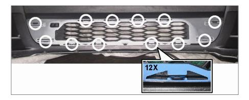
5. Once the lower grille is removed, it will be necessary to modify the existing tab-slots on the front fascia lower grille opening. Mark a cut line along the eight (8) tab slots as shown in the image below. The slots will be cut so they are flush on the inner side of the opening.
