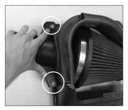
11. Orient the filter so the clamp worm-screw and the filter parting line is viewable from the bottom side of the air box. Tighten the 8mm worm-screw to 3 Nm.
