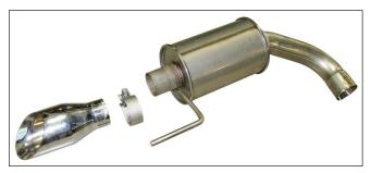
Check the exhaust system for correct clearance under the vehicle and also for tip alignment as shown below. If alignment is off, loosen the required band clamp, adjust, and re-torque the band clamp.
