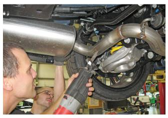
3. With the exhaust pipe cut, slide the hanger out of the rubber mount and remove the muffler/tip assembly from the vehicle.
