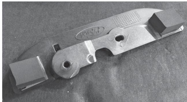
8. Remove the two (2) studs from the factory heat extractors and install them on the ROUSH Heat Extractors.
