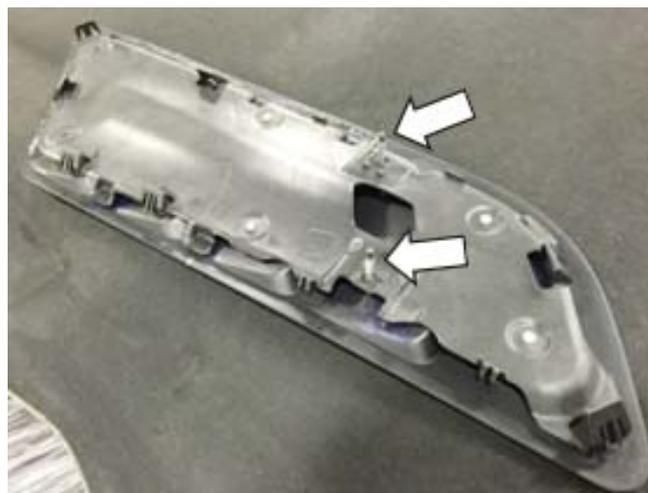
9. Install the ROUSH Heat Extractors by clipping them into the factory slots and installing two (2) T10 screws (P/N: 96817A350) with two (2) washers (P/N: 65120081) in the holes that were drilled in step 6. Torque the screws to 0.4 Nm.
