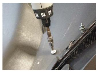
32. Remove the backing off the 2-sided tape, apply blue Loctite® to the threads on the studs that were installed in step 24 and then torque all of the fasteners that were installed in steps 24-26 to 0.7-0.8 Nm.
