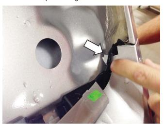
10. Hold the center of the bumper cover and partially remove it in order to gain access to remove the wiring harness connector under the RH tail lamp. With the connector removed, remove the bumper cover and place it on a protective surface.
