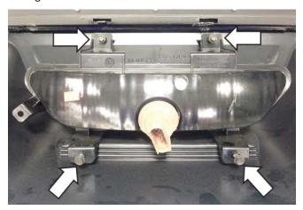
20. Remove three (3) 7 mm screws and three (3) J-clips for the factory rear valance trim piece from each side of the rear bumper cover.
