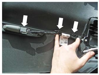
12. Disconnect the license plate light and trunk release electrical connectors as well as the two (2) edge clips that retain the wiring harness.
