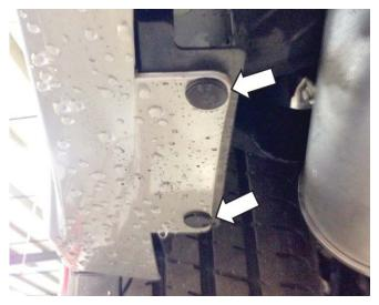
6. Remove two (2) 7 mm screws and two (2) push-in retainers on the LH and RH sides under the rear bumper.
