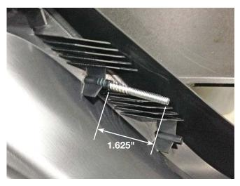
30. Place the rear valance on the bumper cover by first aligning the two outer studs with the lower outer holes drilled in step 21. Loosely install one washer (P/N: 1133153) and one nut (P/N: 90480A011) onto each stud and then lay the back of the rear bumper cover down onto a protective surface
