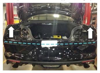
9. Locate and release one (1) retaining tab on each side of the bumper cover near the outer edge of the tail lamp mounting area.
