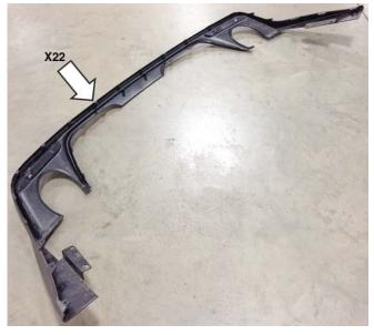
22. Using an air saw, cut and remove the factory lower valance as shown below.
