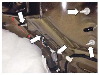
3. Remove three (3) push-in retainers in the back of both rear wheel wells.
