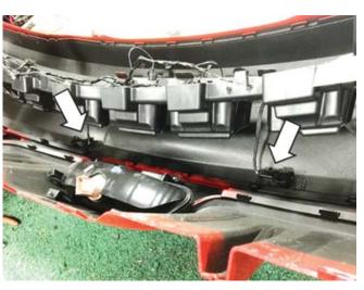
17. Remove the four (4) factory back up sensors by releasing the retaining tabs and then set them in a safe place. Remove the four (4) plastic factory back up sensor brackets from the bumper cover with a suitable cutting tool. Use caution to not damage the factory bumper cover.
