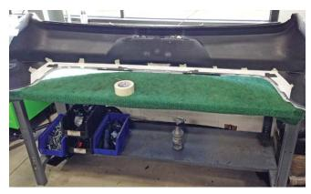
24. Using a 1/8" drill bit, drill fifteen (15) pilot holes and then follow up with the appropriate drill bit as indicated on the template.
