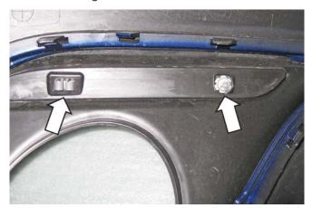
19. Remove the four (4) 7 mm screws for the reverse light.
