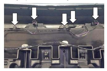
13. Disconnect the reverse light electrical connector as well as the push pin that retains the wiring harness.
