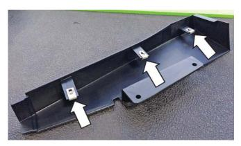
35. Install the side valance pieces onto the rear bumper cover using three (3) screws that were removed in step 17 and completely remove the backing from the 2-sided tape. With the side valance pieces installed press firmly along the back edges to ensure that the 2-sided tape has bonded adequately.
