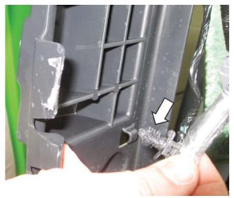
38. Drill a 1/4" hole as shown below, reinstall the push-in retainer and then trim the excess.
