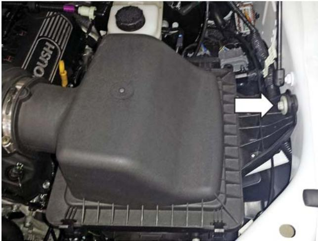
4. Loosen the hose clamps retaining the clean air tube to the throttle body and air box lid.
