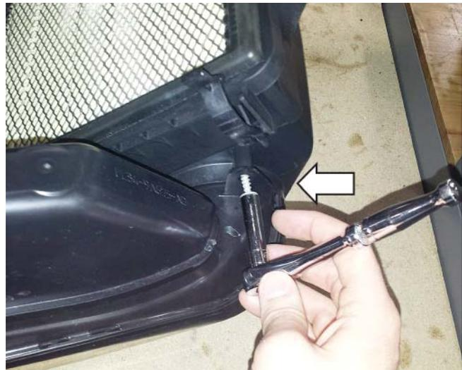
12. Remove the dirty air inlet from the lower air box.
