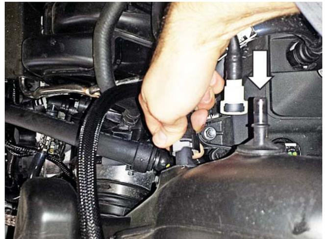
6. Release the two (2) clamps on the front of the air box.
