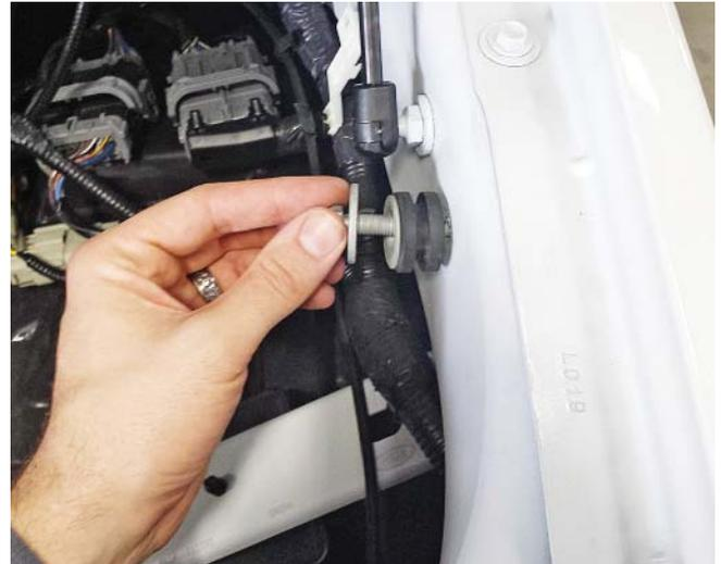
13. If necessary, remove the two (2) rubber grommets from the bottom of the air box and reinstall them into the tray below the air box.
