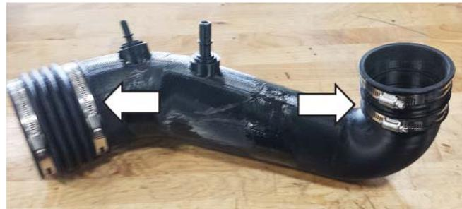
9. Install the clean air tube assembly between the throttle body and the air box. Tighten the clamps to 3 Nm.
