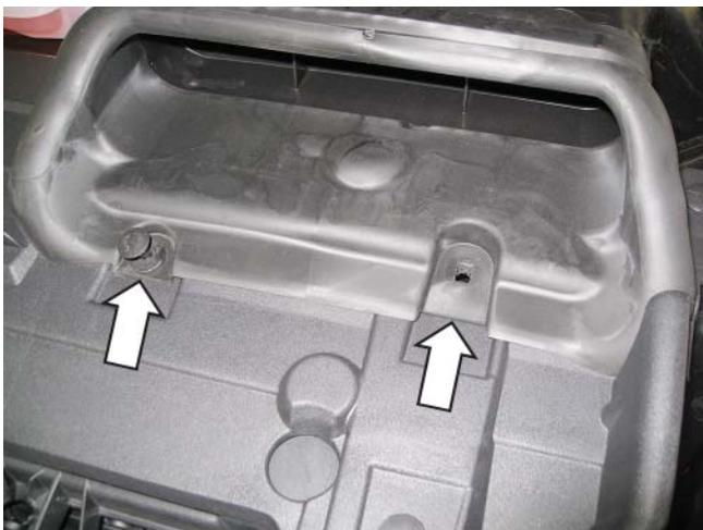
12. Insert the seal filler (P/N: 1115-9B624FOAM) halfway into the air box seal (P/N: 1115-9B624) as shown.
