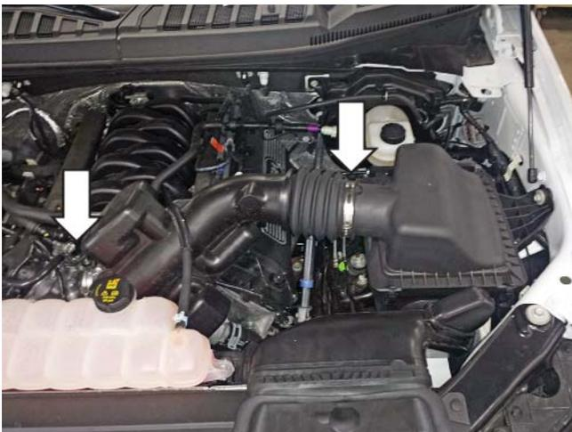
5. Disconnect the two (2) quick connect fittings from the clean air tube.
