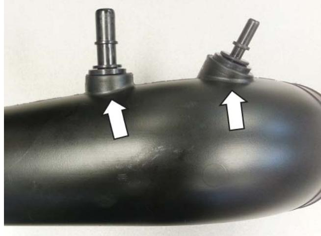
8. Install couplers and clamps onto the clean air tube (P/N: 111550-9B660) as shown. Tighten the clamps retaining the coupler to the tube to 3 Nm. Leave outside two (2) clamps loose (couplers: right P/N: 111550-9B662, left P/N: 111550-9B662) (clamps: right P/N: R07130015-13, left P/N: 308707426).
