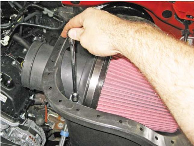
7. Install the rubber grommet (P/N: 1150-58GRMT) and fittings into the clean air tube. You will want to use soapy water or glass cleaner to aid the installation (fittings: left P/N: 1311-9N285, right P/N: KLR-9N285).
