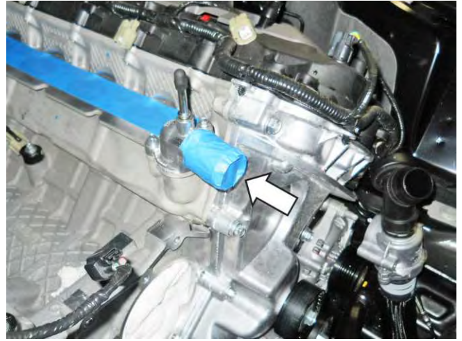
61. Tape off and block the thermostat housing ports. Use care to prevent coolant from leaking from the housing and hose.
