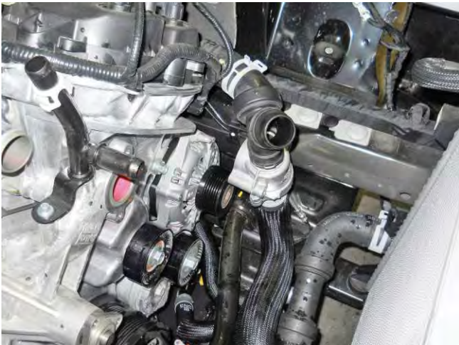
57. Remove the four (4) water pump mounting bolts (10 mm socket) and remove the water pump. Set both aside for re-use.
