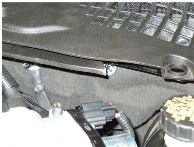
Exposed point on modified K-brace, shown installed
