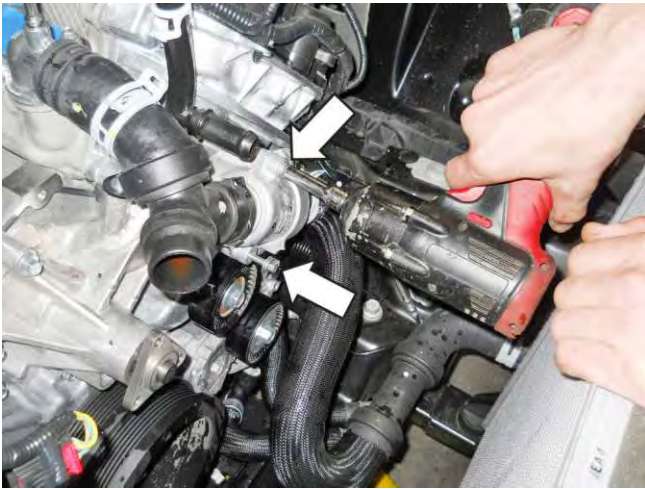
56. Remove the thermostat housing assembly and set it aside.
