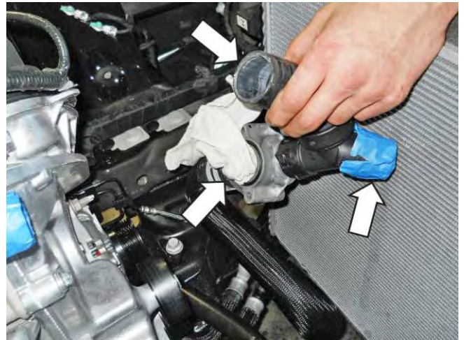
61. Tape off and block the thermostat housing ports. Use care to prevent coolant from leaking from the housing and hose.
