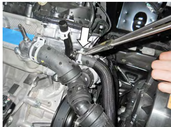
Degas hose from bottom of bottle
