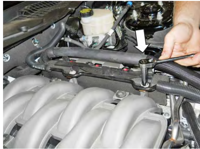
32. Disconnect the brake boost vacuum hose from the port at the firewall.
