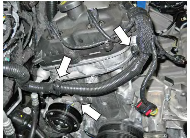
54. Loosen the clamp and disconnect the coolant hose, at the outlet neck.
