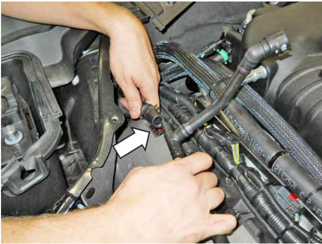
45. Connect the PCV purge line (13116K817) to the PCV valve on the RH cam cover and the port on the RH side of the supercharger.
