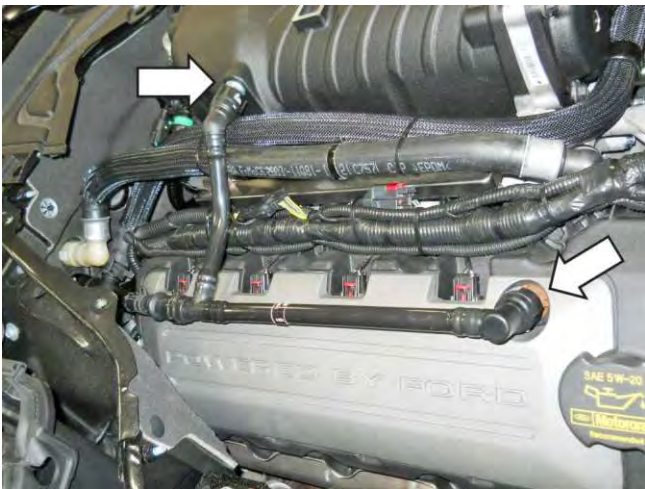
45. Connect the PCV purge line (13116K817) to the PCV valve on the RH cam cover and the port on the RH side of the supercharger.
