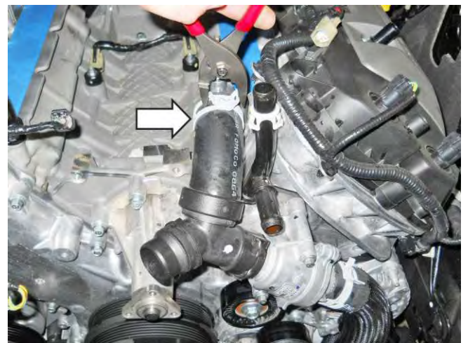
55. Remove the two (2) bolts from the thermostat housing (8 mm socket).
