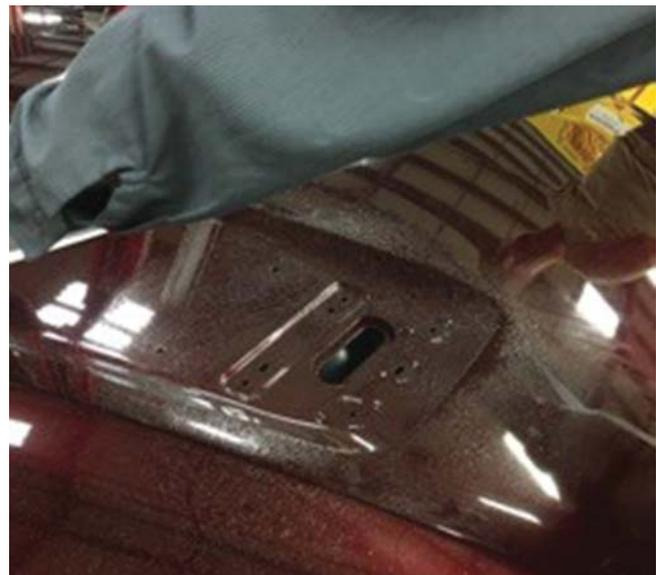
8. Align the holes in the graphic to the holes in the hood and lay the graphic (P/N: 1318-16C829LH and 1318-16C830RH) onto hood, applying the graphic top down as shown. Using a plastic applicator, work out larger bubbles in the graphic by pushing them to the outer edges. Pop smaller bubble with a razor blade or pin.
