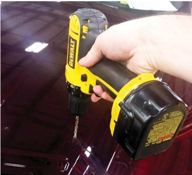
6. On the underside of the hood, drill a 1-inch hole in the inner structure using the previously drilled 1/8" hole as a pilot hole. **IMPORTANT: DO NOT DRILL A 1-INCH HOLE IN HOOD SKIN!** Once the holes are drilled, apply commercially available clear coat (Motorcraft P/N: PM-19500-6000) to the exposed metal so that it does not oxidize. Repeat on opposite side.
