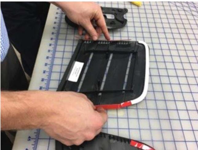
12. Remove remaining backing off double-sided tape and apply the heat extractor to the hood. Apply even pressure all around perimeter to wet out tape fully.
