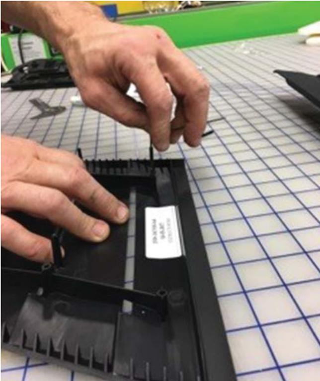
11. Clean the back side of the heat extractors with an isopropyl alcohol and water mix. Remove one (1) side of the backing of the double-sided tape, two (2) pieces of P/N: 1318-16C925 and one (1) piece of P/N: 1318-16C926 for each extractor, and place onto the outer ribbing as shown. Repeat on other side.
