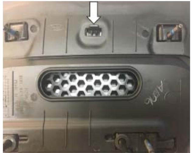
4. Cut out the drill templates (P/N: 1318-16C929TMPL and 1318-16C930TMPL) from the last pages of this instruction manual. **(IMPORTANT:** Print template to scale. Check scale by measuring reference line with a ruler.) Align black outlined holes with factory holes (using a pen or center punch as shown is helpful). Tape the templates in place and then mark the two (2) drill holes with a center punch. Repeat on other side.
