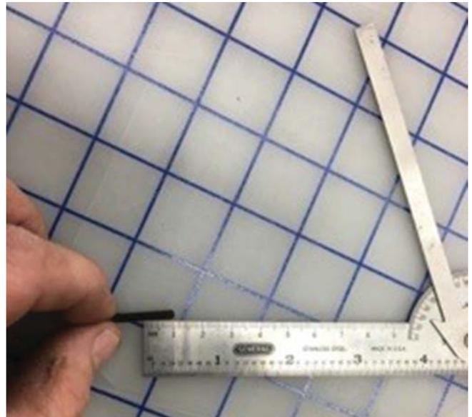
10. Hand start each stud (P/N: 25112) in the heat extractors (P/N: 1318-16C929 and 1318-16C930). Use a 1/16" Allen key to tighten each stud down to the mark made previously. You should have 22 mm of stud protruding.
