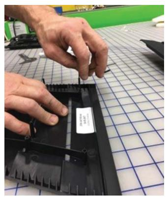
Clean the back side of the heat extractors with an isopropyl alcohol and water mix. Remove one (1) side of the backing of the double-sided tape, two (2) pieces of P/N: 1318-16C925 and one (1) piece of P/N: 1318-16C926 for each extractor, and place onto the outer ribbing as shown. Repeat on other side.
