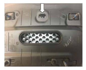
Cut out the drill templates (P/N: 1318-16C929TMPL and 1318-16C930TMPL) from the last pages of this instruction manual. (IMPORTANT: Print template to scale. Check scale by measuring reference line with a ruler.) Align black outlined holes with factory holes (using a pen or center punch as shown is helpful). Tape the templates in place and then mark the two (2) drill holes with a center punch. Repeat on other side.
