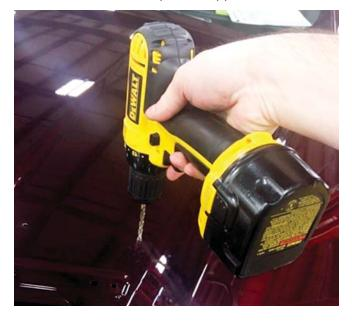
On the underside of the hood, drill a 1-inch hole in the inner structure using the previously drilled 1/8" hole as a pilot hole. **IMPORTANT: DO NOT DRILL** A 1-INCH HOLE IN HOOD SKIN! Once the holes are drilled, apply commercially available clear coat (Motorcraft P/N: PM-19500-6000) to the exposed metal so that it does not oxidize. Repeat on opposite side.
