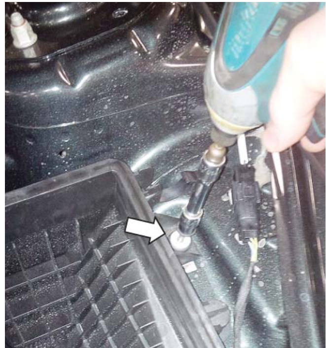
10. Remove the air box tray and dirty air inlet from the vehicle.
