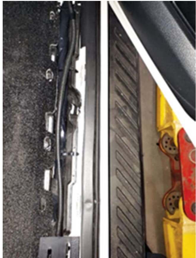
20. Remove the sill plate from the passenger side floor by firmly pulling up.
