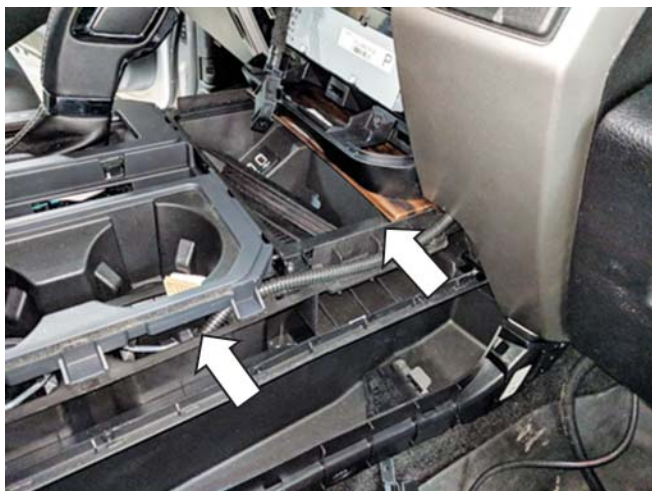
16. Mount the active exhaust on/off switch in the desired location as shown.
