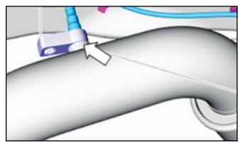
2. Remove the three (3) bolts from the flange securing the over axle pipe to the DPF flange (15 mm).
