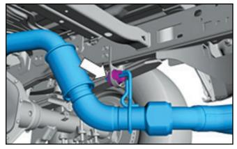
5. Remove the factory exhaust gasket.
