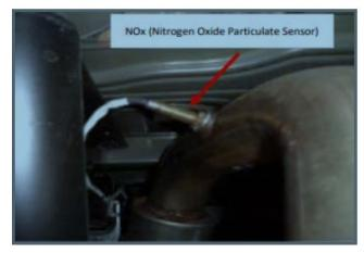
2. Remove the 3 flange nuts at the upstream end of the tailpipe assembly with a15mm socket. (Don't discard the nuts or bolts, they will be reused in the new exhaust installation process)
