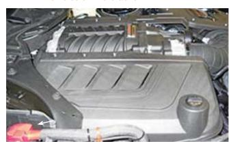
Install three (3) 18-8 button-head socket capscrews (92095A240) on the cover and torque to 7 Nm.
