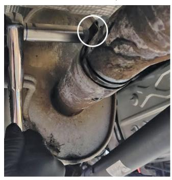
Remove the front exhaust hanger from the vehicle side and then remove it from the factory exhaust. Set aside.
