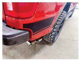
7. Starting from the front of the vehicle and working toward the back, tighten the clamps to 55 Nm, ensuring that the tips remain aligned.
