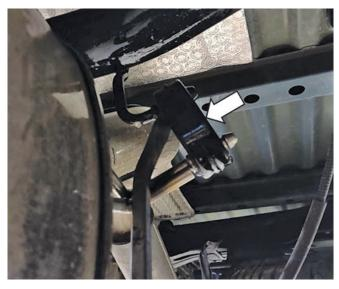
5. Lower the exhaust system and remove it by pulling it out of the last remaining hanger.
