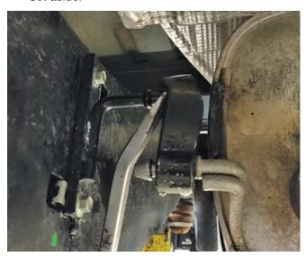
4. Remove the rear exhaust hanger over the top of the axle and then remove it from the factory exhaust. Set aside.
