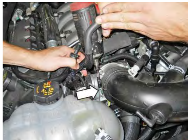
Clamp at throttle body
