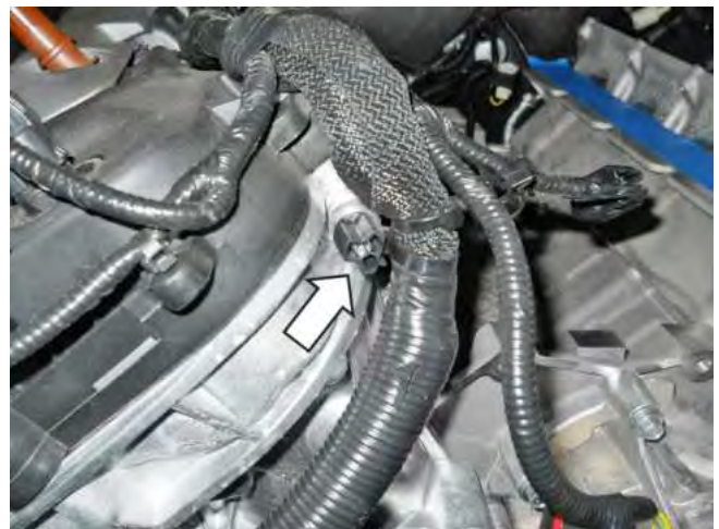
44. Unclip the engine electrical harness retention clips that retain the engine harness to the top corners of the RH (passenger side) front cover.
