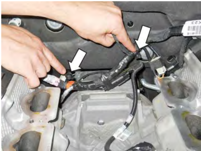
Pin retainers on harness
