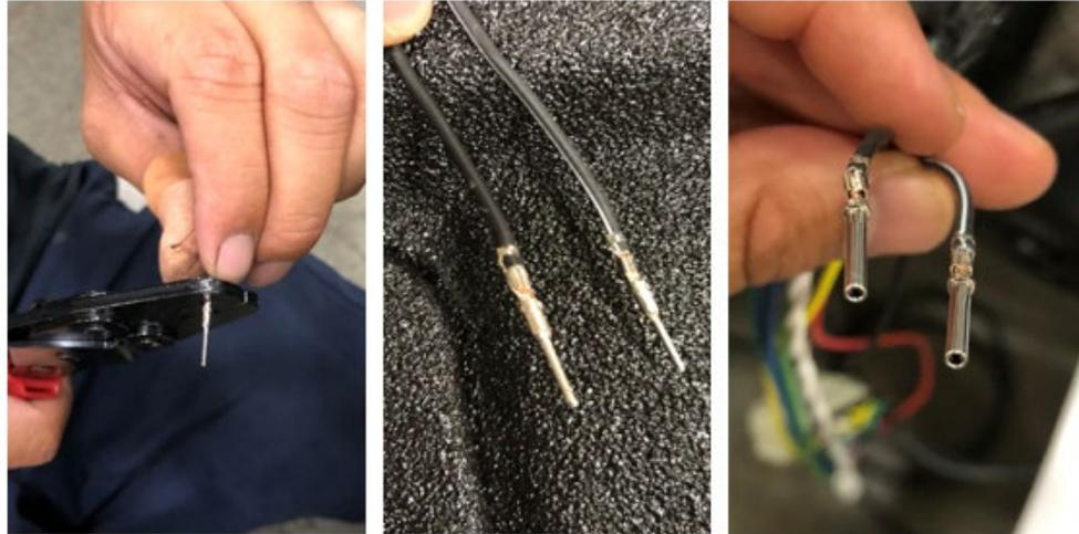
12. Install the newly connected pins from each half of the harness into the two (2) supplied electrical connector shells taped to the wire harness.
