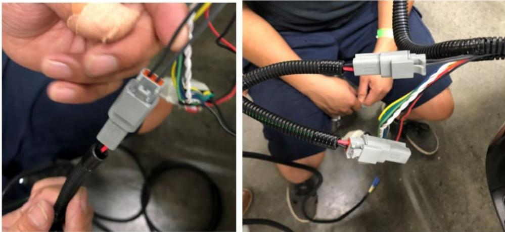
14. Zip tie and tape the harness together. Re-attach the electrical connector to the taillight and re-install the taillight using the two (2) screws previously removed. Torque to 5 Nm.
