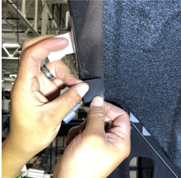
5. Install the spring clip over the tape as shown.
