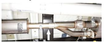
13. Install the takeoff hanger as shown onto the 3" over-axle pipe (PT00038892).
