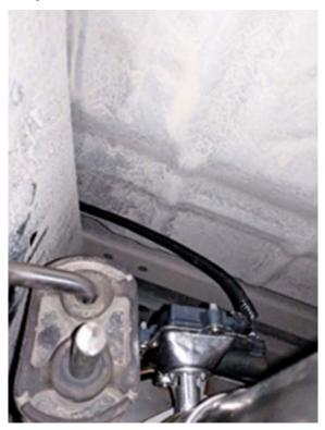
20. From inside the cab, pull gently on the wire until all slack is taken up. Use a zip tie to secure the wire to the wall of the cab. Zip tie the relay to the rear wall of the cab.
