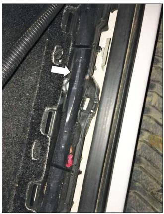
15. Loosen the B-pillar trim piece by pulling just below where the seat belt comes out. Do not remove.
