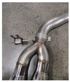
15. Slide a 3" clamp (10-0439) on the tip and slide onto over-axle pipe(PT00038892). Install the hanger onto the passenger side frame rail with the over-axle exhaustpipe and tip attached.
