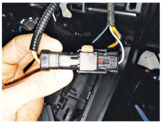
9. Plug the 12V and 110V connectors into the trim panel and leave loose. (The switch can be installed next to the power port if the vehicle doesnot have the 110V power source)
