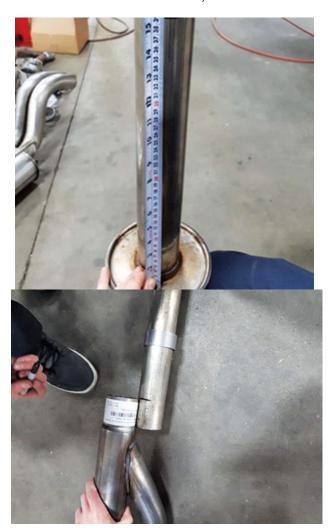
Using the supplied gasket (CV6Z-9450-C) and two (2) nuts (NM8X125HF-S437), install the exhaust valve (PT00042392) onto the muffler (PT00038572) as shown. If installing the PASSIVE system, use two Gaskets (CV6Z-9450-C) and the outlet adapter (1315-5232CPL) Torque the nuts to 25 Nm.
