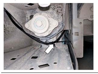
19. Plug the connector into the valve on the muffler.
