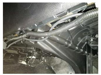
13. Secure the harness (CTUV740) up under the dash using the supplied zip ties.
