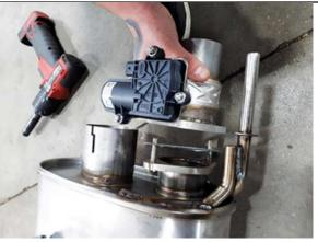
7. Slide a 3" clamp (10-0439) over the Y-pipe (near the flex joint). Slide a 2.5" clamp (10-0338) over the other two (2) joints. Install the Y-pipe onto the factory resonator pipe as shown.
