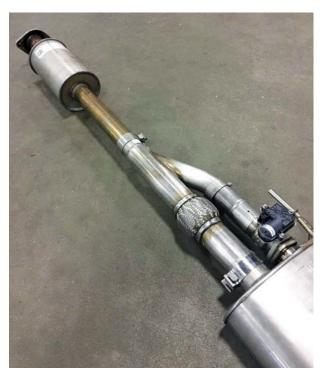
9. Install the mid-bed isolator onto the bed. Torque to 25Nm. (10mm Socket).
