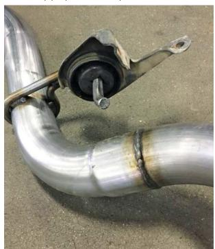
14. Install the supplied hanger (1115-5A204) onto the dual exhaust tip (PT00038638).
