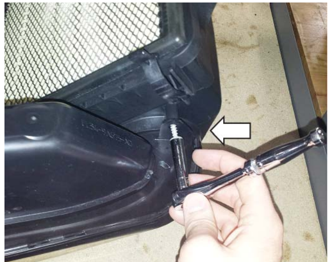
11. Remove the self-tapping screw retaining the dirty air inlet onto the lower air box.
