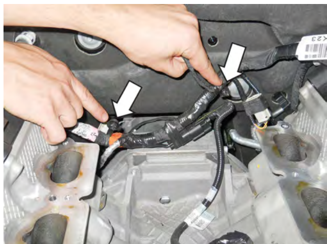
Pin retainers on harness
