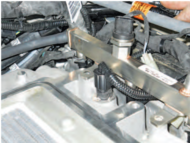
12. Lubricate the lower fuel injector O-rings with petroleum jelly or engine oil. Install the fuel rail and injectors into the intake manifold. Be sure each injector is properly seated into the intake manifold.
