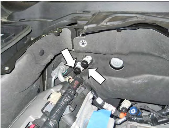
46. Tape off the radiator hose port and inlet port.
