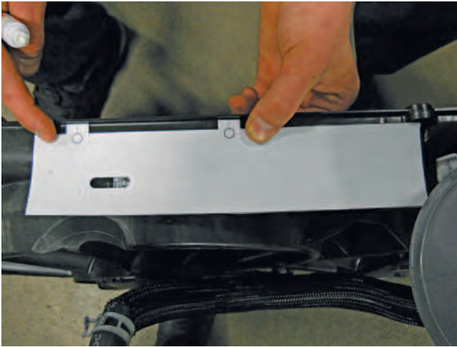
Proper template position on fan shroud
