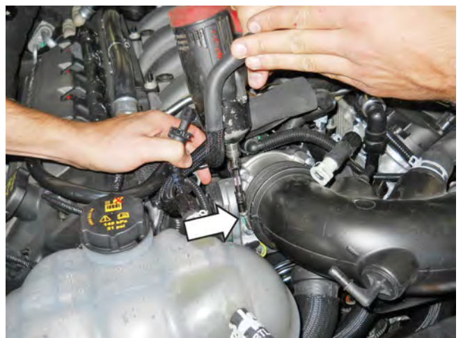
Clamp at throttle body
