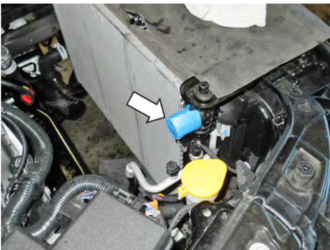
46. Tape off the radiator hose port and inlet port.
