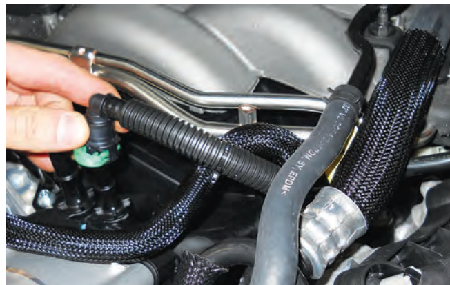
EECPV tube quick connector with green lock
