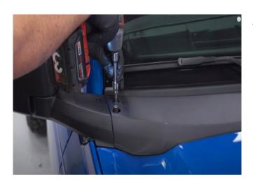
3. Lift cowl after four bolts have been removed, Open vehicle hood.
