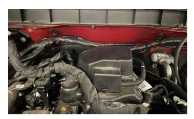
Verify the length for connectors thru the openings by the hood hinges, up thru the panels above and to the lights, use edge biter clip zip ties on both driver's side and passenger's side as circled below, cut off the end of zip ties to desired length.
