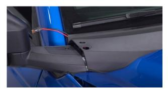
6. While working on the passenger's side, align the Work Light Mounting Bracket in position as shown, tighten down the T25 torx fastener with the supplied washer from the kit.
