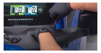
8. Locate one LED light pod, Position the two 5/16 nuts in the holes located at the back of the light pod. (The two nuts are facing toward each other)
