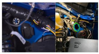
2. Fish wire and switch thru hole and into interior. Be sure to have enough wire going into the interior to reach the desired switch location.
