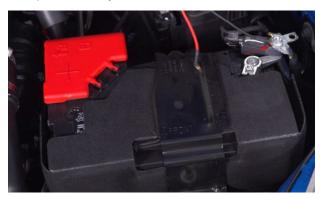
9. Open red protective cover over battery positive terminal and install red positive wire to bus bar terminal using one of the fasteners on the bus bar.
