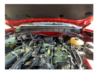
3. Zip ties the given wiring harness to the existing wire at the back engine compartment wall as example shown below, cut off the end of zip ties to desired length.
