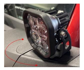
3. Examples below shows the light direction (red arrows) in either center position or side position.
