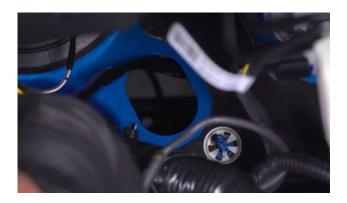
3. With the on/off switch wires in, reinstall the plug from the interior side working around the harness.
