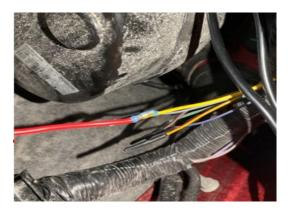
6. Connect the black ground wire and fasten it with 8mm socket to the existing ground on the driver's side rear cowl area. 7. Add zip ties as shown below to make the engine bay organized.
