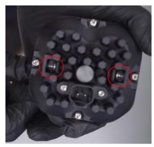
9. Use the two 5/16 allen screws secure the lamp to the driver side Work Light Mounting Bracket
