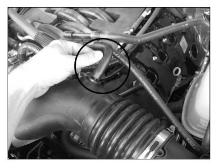
18. Connect the PCV line fitting onto the port in the clean air tube.
