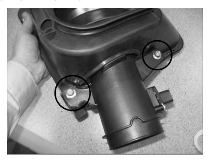
14. Orient the filter so the clamp worm-screw and the filter parting line is viewable from the bottom side of the air box. Tighten the 8mm worm-screw to 3 Nm.
