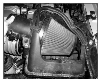
16. Install the new clean air tube between the throttle body and the new ROUSH air box lid assembly. Secure the clamps for the air box lid and tighten both clamps on either end of the clean air tube. Torque the clamps to 3 Nm.
