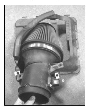
12. Install the EPDM close out seal (1111-9645) around the MAF Tube and clip into the edges of the upper air box tray.
