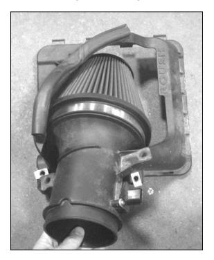
11. Install the EPDM close out seal (1111-9645) around the MAF Tube and clip into the edges of the upper air box tray.
