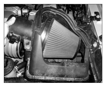
15. Install the new ROUSH clean air tube between the intake and the new ROUSH air box lid assembly. Secure the clamps for the air box lid and tighten both clamps on either end of the clean air tube.
