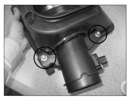
13. Orient the filter so the clamp worm-screw and the filter parting line is viewable from the bottom side of the air box. Tighten the 8mm worm-screw to 3 Nm.
