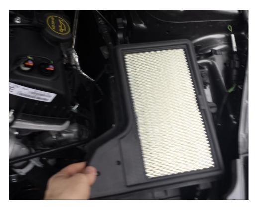
7. Remove the bolt holding the air box to the inner fender using the 10mm socket.
