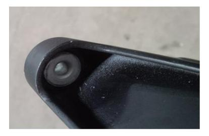
2. Install the second grommet onto the air box (131550-9A612).
