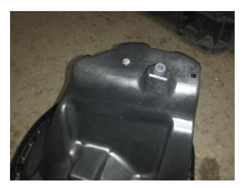
4. Insert the dirty air inlet (1315-9F763-A) into the air box (131550-9A612).
