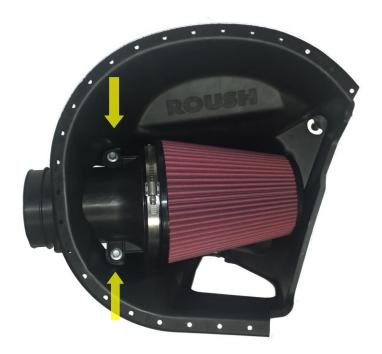
13. Install the clean air tube coupler onto the turbo inlet (Part Number 131523-SILCP-AA) and tighten clamp (Part Number 5340). Use clamp (Part Number 5348) to fasten the clean air tube to the coupler. Lastly tighten the clamp from the clean air tube to the air filter tube (Part Number R07130028-13-AA). Tighten clamps to 3 Nm.
