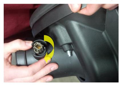
14. Connect the temperature sensor connector.
