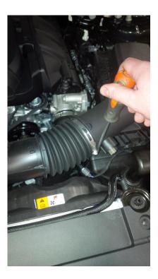
5. Release the two latches holding the air box lid to the lower box.
