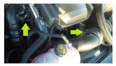
16. Install the PCV tube with the quick connect (make sure it's fully seated), followed by the recirculation valve hose with the constant tension clamp.
