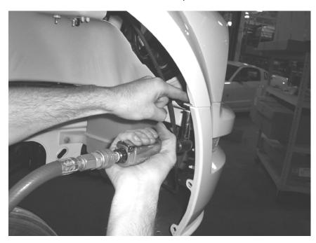
7. After all hardware has been removed, carefully remove front fascia from car by pulling the top corner down off of bolts. (Figure F)
