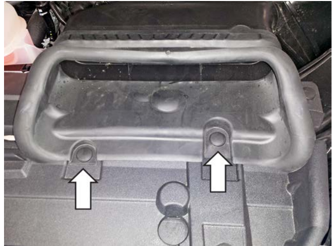
10. Remove the lower air box and dirty air duct from the vehicle.
