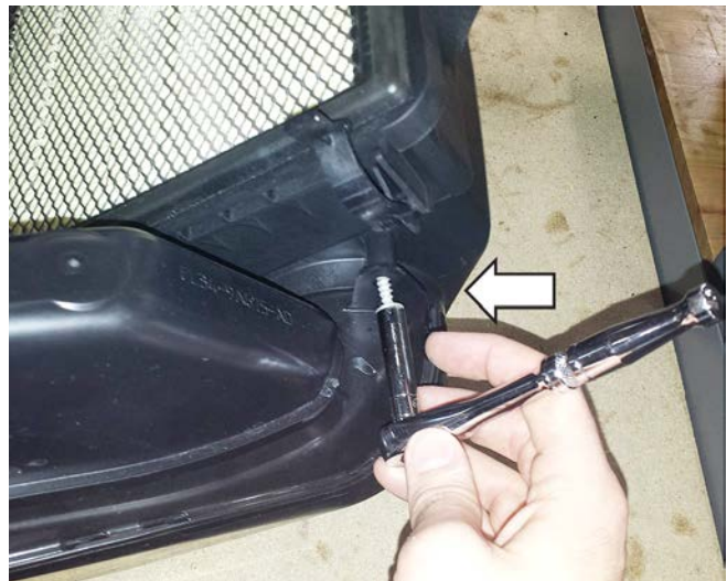
11. Remove the self-tapping screw retaining the dirty air inlet onto the lower air box.
