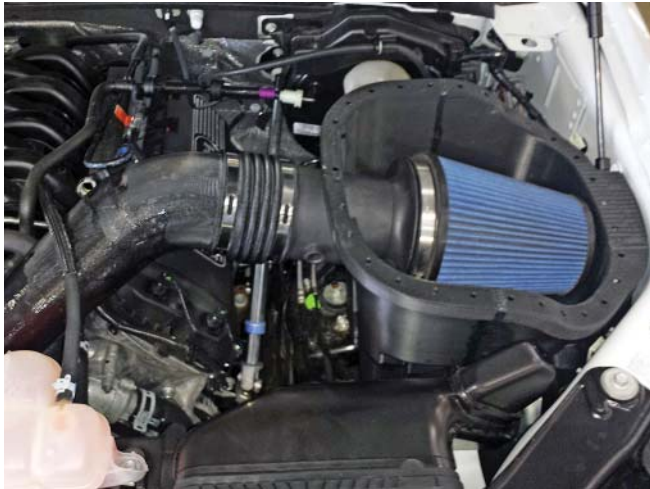
10. Attach the two (2) quick connect hoses to the mating bars on the clean air tube.
