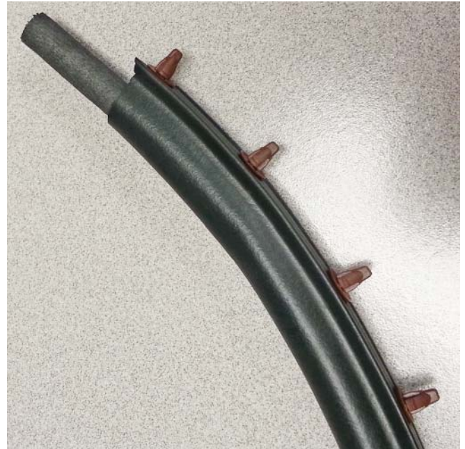
13. Install the air box seal starting in the location shown. You may need to trim the seal to the correct length. (Note: Start the seal at the middle of the inlet tube.)
