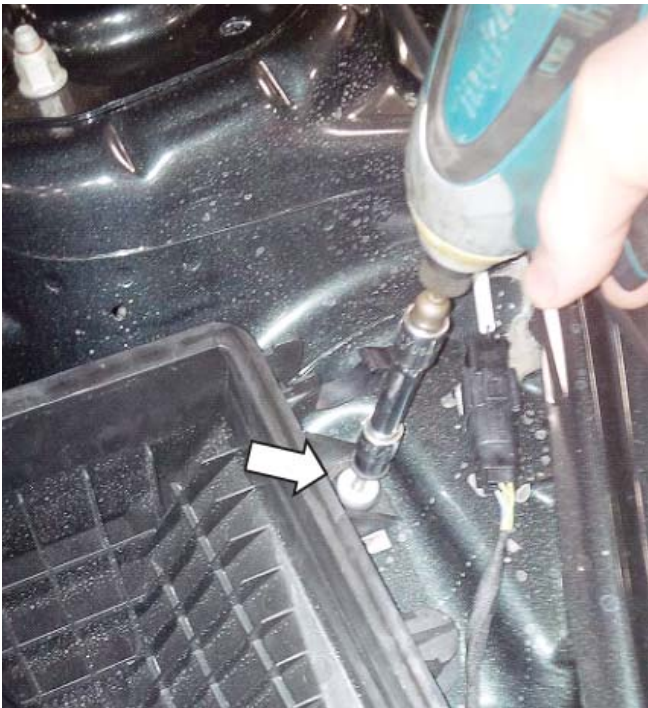
8. Remove the air box tray and dirty air inlet from the vehicle.
